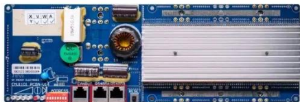
BS4S Communication between battery and inverter Band rate:9600bps BS4S Interface Communication between parallel packs of BMS and PC Band rate:9600bps
